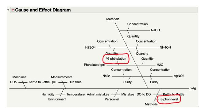
Operators had been taught to siphon as much supernatant liquid as possible. The coagulated gel had variable density. It was better to siphon to a standard level than to siphon as much as possible
