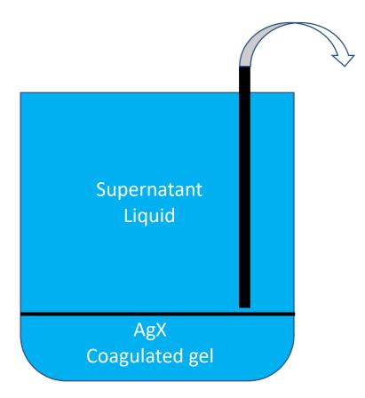
To wash out the nitrate, sodium, and potassium ions. Acid is added to coagulate the gel. The supernatant liquid is drawn off with a siphon.
