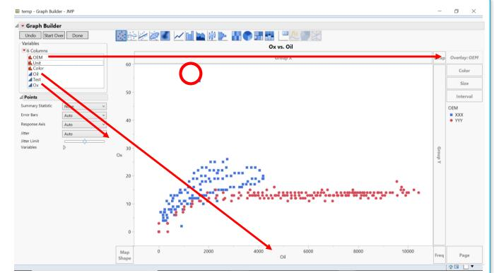
Engine oil oxidation – "Oil hours" vs. "Test hours"
