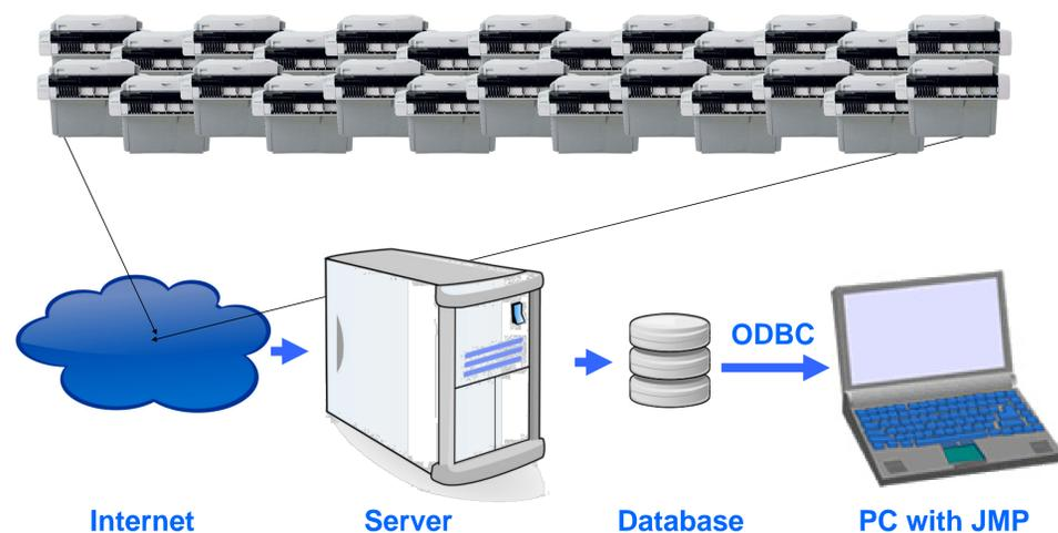
Data from instruments worldwide is collected in a database without patient identifying information. The database can be accessed with JMP through an ODBC connection. Using a combination of JMP interactive menus and JMP scripting both product performance and customer behavior can be evaluated.
