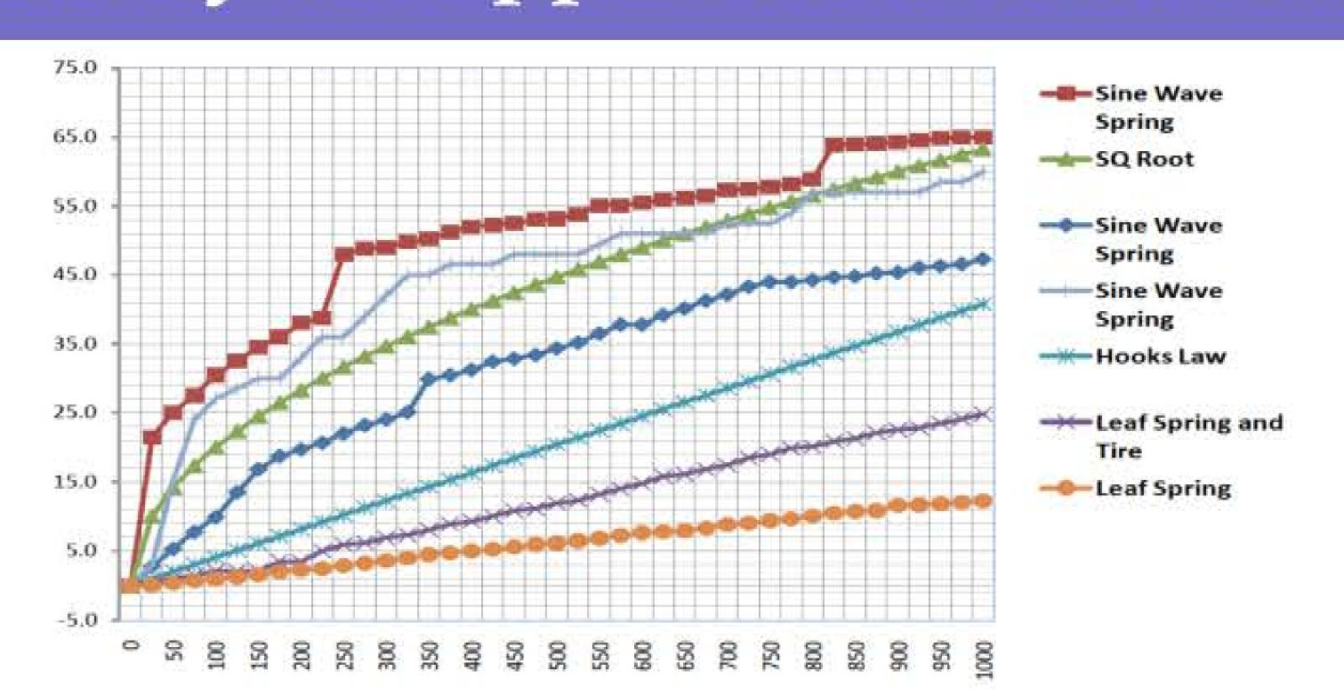
Load Test results of a Sine Wave Spring as compared to the performance of a normal leaf spring and tire. The graph shows the superior low and high end performance of the sine wave spring. Baseline projections are shown by the "SQ Root" and "Hooks Law" line for the two types of springs.
