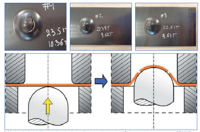
Crédit photo: Application of laser speckles to localized necking and cracking detection in Erichsen cupping test, CEZARY JASI¡SKI, ROK WYD. LXXIII, ZESZYT, 9/2014
